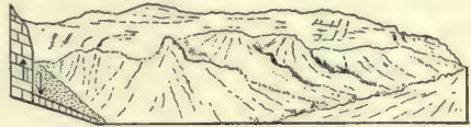
FIG. 63.—Fault scarp in Arizona. Land waste has accumulated at the base of the scarp and conceals the lower part. The diagram shows the structure. (Ransome, U. S. Geological Survey.)
